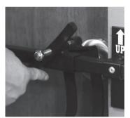
**STEP 3:** Spin the turn handle until the locking device is tightly secured on the door.
