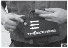
**STEP 1:** Door closers are adjustable for different size closers. Adjust the bolt to one of the three holes to ensure a snug fit on the door closer.
