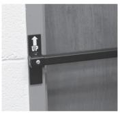
**STEP 2:** Position the bar so that the foot pad rests against the face of the door jamb.
