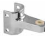
TOP HINGE 1-1/8" Bet. Screws For 1-1/4" Rnd. Post Part No. 96320A A = 1-11/16"
