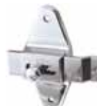
SLIDE BOLT LATCH 3-1/2" Between Screws 3/8" Door to offset bar clearance Part No. 9G0137 - Chrome Part No. 9A5063 - Cast Stainless Steel
