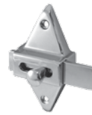
SLIDE BOLT ASSEMBLY 2-3/4" Bet. Screws 9/16" Bar to Door Clearance Part No. 9F0302
