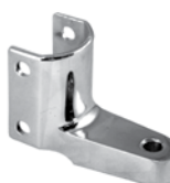
BOTTOM HINGE 1-1/8" Bet. Screws For 1-1/4" Rnd. Post For 9KCAMM & 9K0231 Part No. 9K0230 A = 1-11/16"
