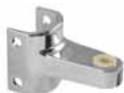
TOP HINGE 1-1/8" Bet. Screws For 1-1/4" Rnd. Post Part No. 9K0240 A = 1-11/16"
